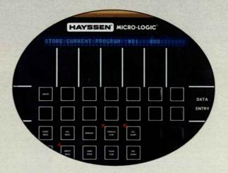
... standard MICRO-LOGIC® microprocessor-based machine control system which allows digital settings to be programmed for up to 32 package sizes and instantly recalled by a single touch of its keyboard ...
