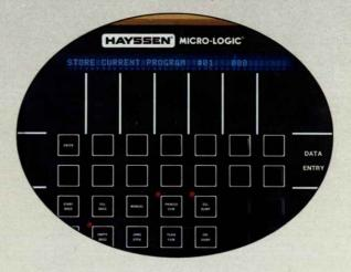
... standard MICRO-LOGIC® microprocessor-based machine control system which allows digital settings to be programmed for up to 32 package sizes and instantly recalled by a single touch of its keyboard . . .
