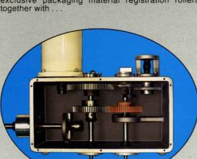
A rugged, totally enclosed oil bath gear box transmits power to the registration rollers and continuous motion belts and provides timing signals through a rotary encoder to either the . . .
