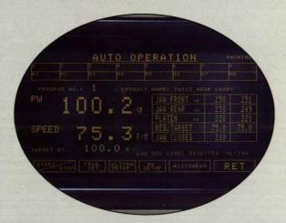
... or the optional MACRO-LOGIC® microprocessorbased total machine (bag maker and scale) control system offering 100 program storage capability, a touch-screen display, a self-contained automatic temperature control system, and an available bar code reading system.
